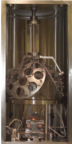
Chamber showing Knudsen Planetary and Electron Beam Gun
